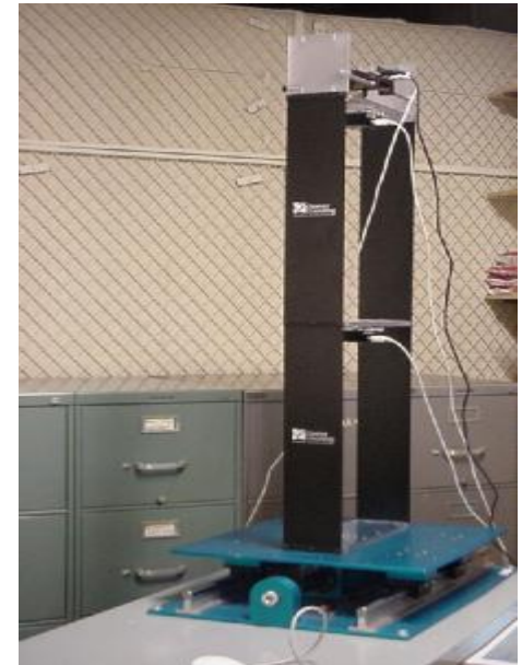
Shake table ( Civil Eng. , to be deployed early 2004 )
